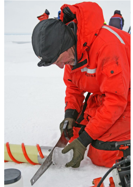
Sawing through an ice core to obtain samples to study climate change. Photo credit: Flickr user NOAA Photo Library.
