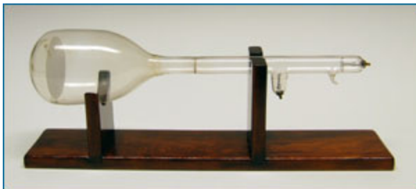
A cathode ray tube from the early 1900s.
